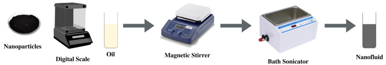
Figure 2: Two-step production approach used to fabricate the nanolubricants of different concentrations.
