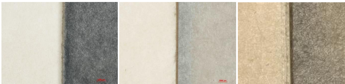
Figure 1. Grey coloration of Nomex® 410 seen after exposure to R-1233zd(E) and MO (left), after exposure to R-454B and POE (center), and after exposure to R-1234yf and POE in AHRI MCLR Project #08007 (right). An unexposed sample of Nomex is on the left in each photo for reference.
